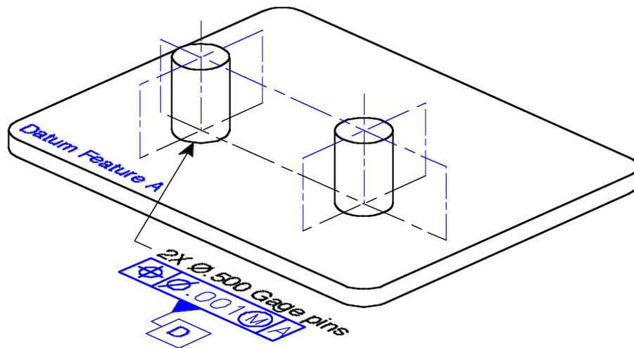
**Figure 4-2C** The three mutually perpendicular intersecting datum planes of a simulated datum reference frame consisting of a plane and two cylinders.
