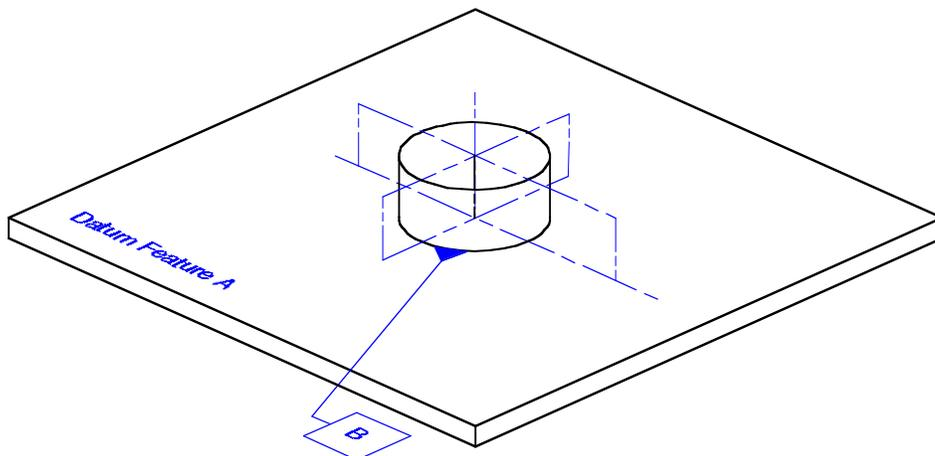
**Figure 4-2A** The three mutually perpendicular intersecting datum planes of a simulated datum reference frame consisting of a plane and a cylinder.
