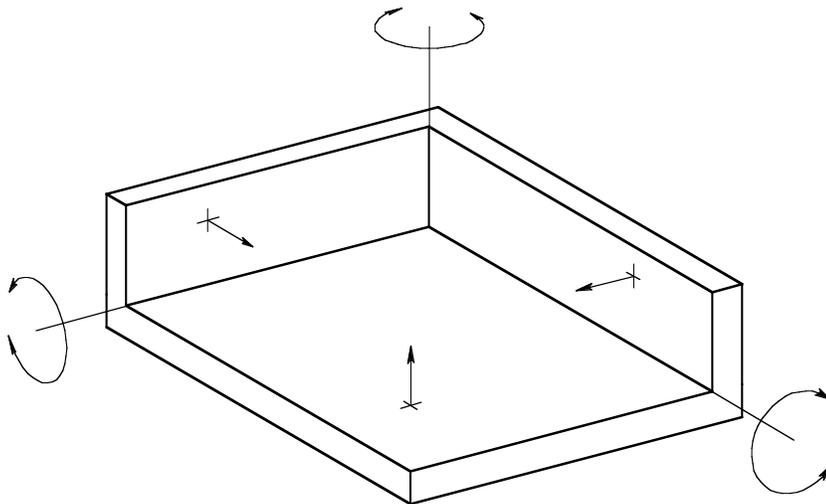
**Figure 4-1** The three mutually perpendicular intersecting datum planes of a simulated datum reference frame.
