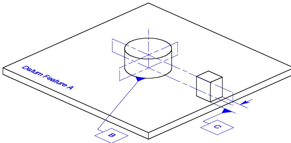
**Figure 4-2B** The three mutually perpendicular intersecting datum planes of a simulated datum reference frame consisting of a plane, a cylinder, and a key.
