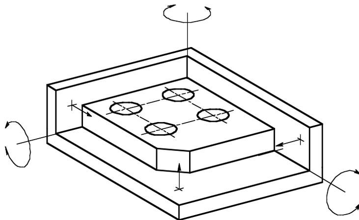
**Figure 4-2** Immobilizing a part within the three mutually perpendicular intersecting datum planes of a simulated datum reference frame.
