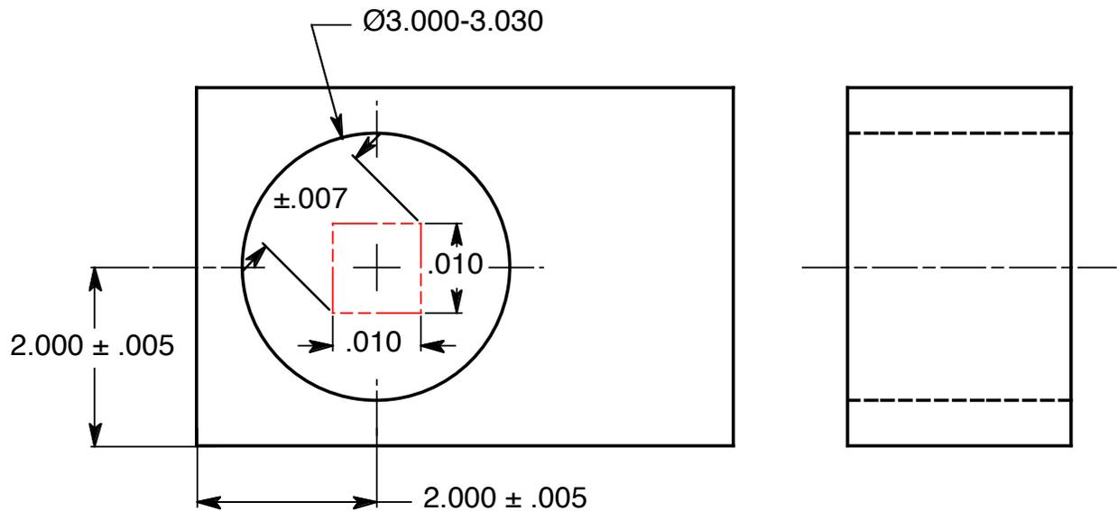
**Figure 1-1** The traditional plus or minus tolerance zone
