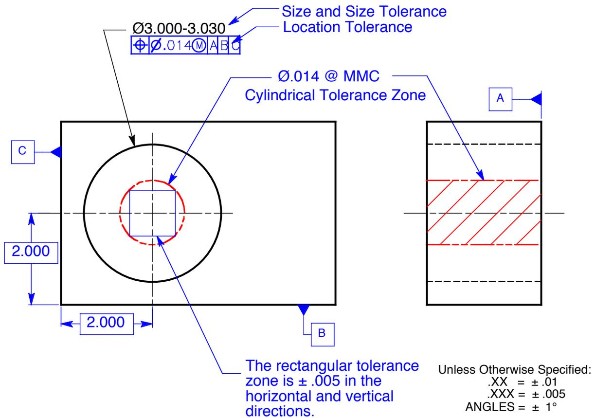
**Figure 1-2** The rectangular tolerance zone converted to a cylindrical tolerance zone
