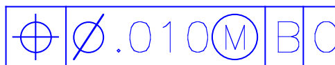
Figure 14-3 A feature control frame with a position tolerance locating and orienting the hole to the primary and secondary datum features - datum features B and C
