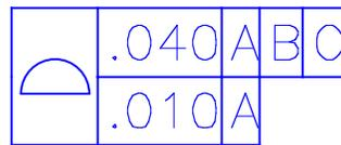
**Figure 12-14A A composite profile feature control frame**
