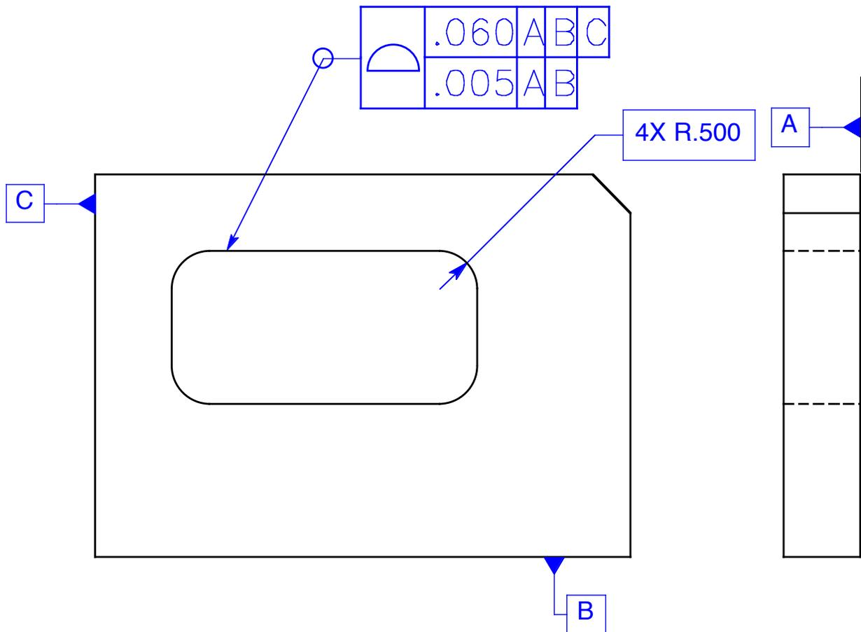
**Figure 12-16 A composite profile tolerance with two datum features repeated in the lower segment of the feature control frame**
