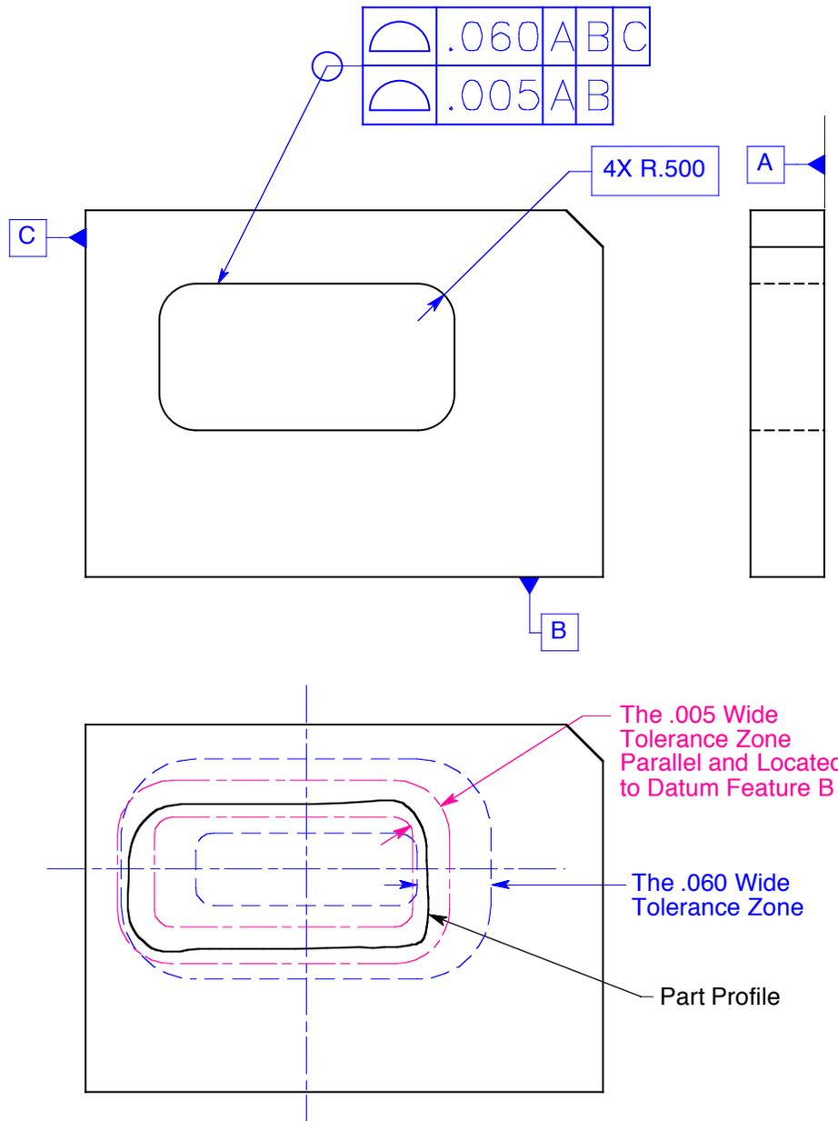
**Figure 12-17 A multiple single-segment profile tolerance**
