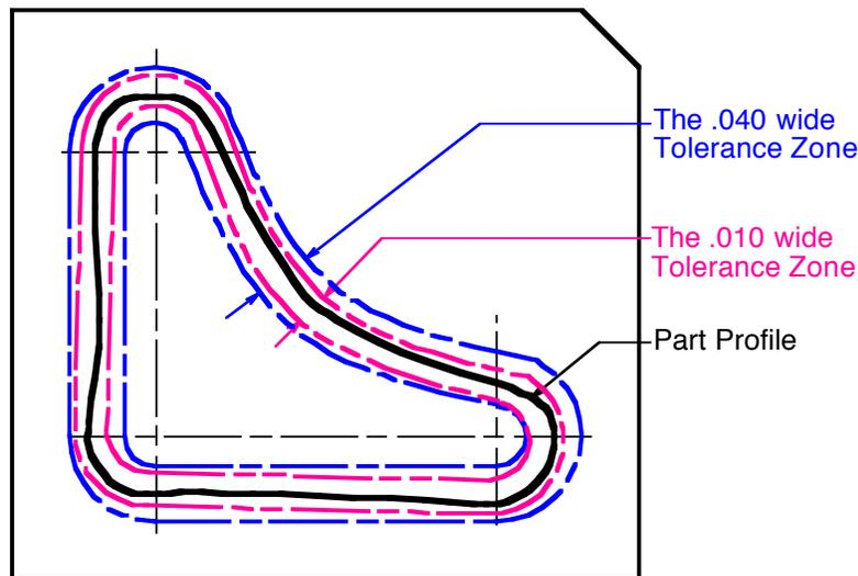
**Figure 12-14 A feature controlled with composite profile tolerancing**
