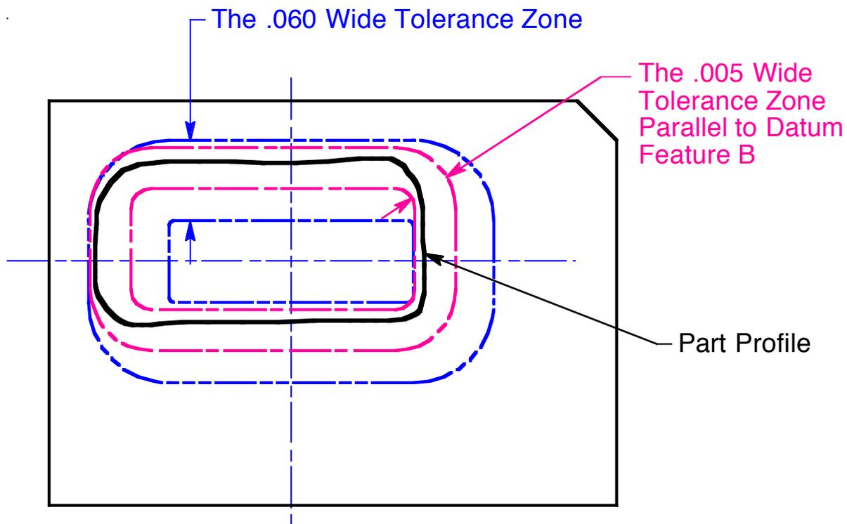
**Figure 12-16A Two tolerance zones generated by the composite profile tolerance with two datum features repeated in the lower segment of the feature control frame**
