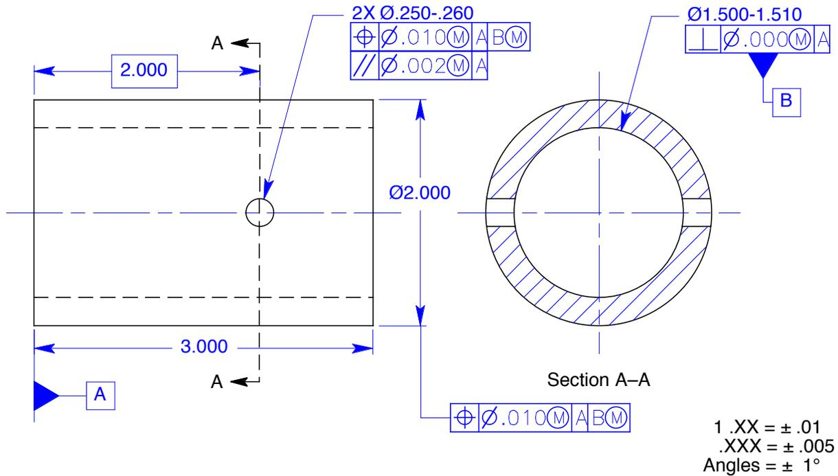
**Figure 9-12 The part in figure 9-11 more completely toleranced**
