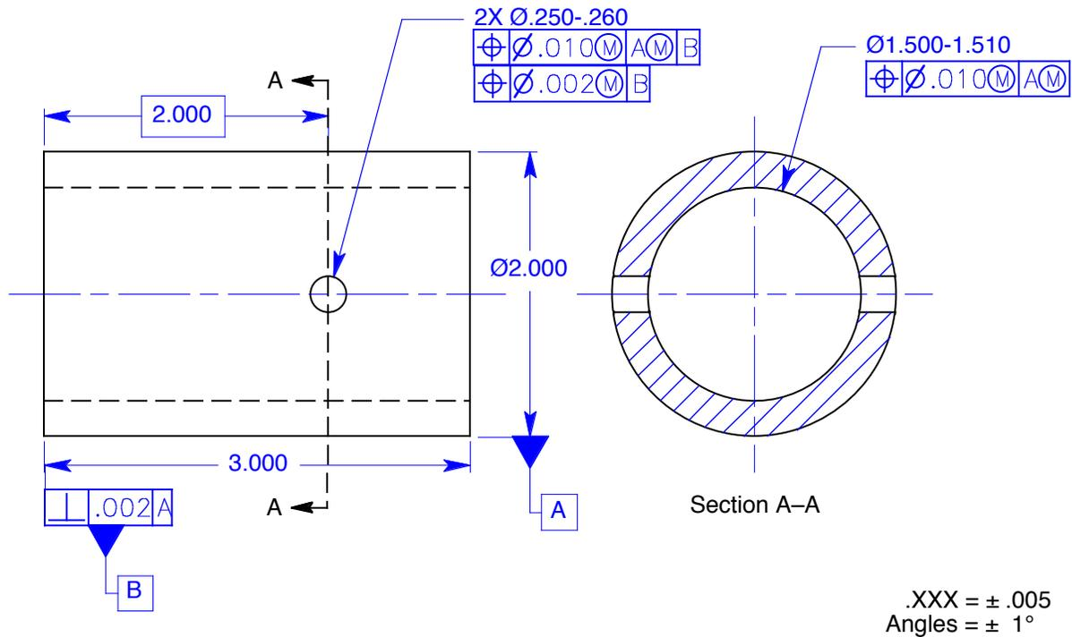
**Figure 9-14 A third method of tolerancing the part in figure 9-11**
