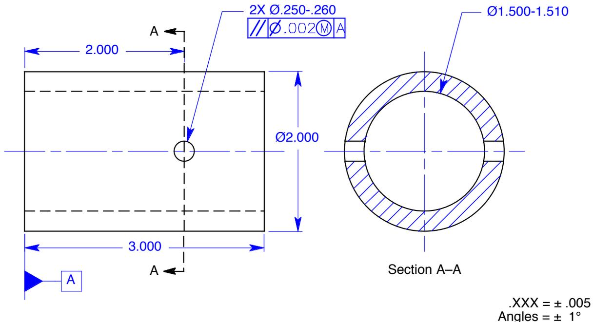
**Figure 9-11 A client drawing specifying the location of two holes**
