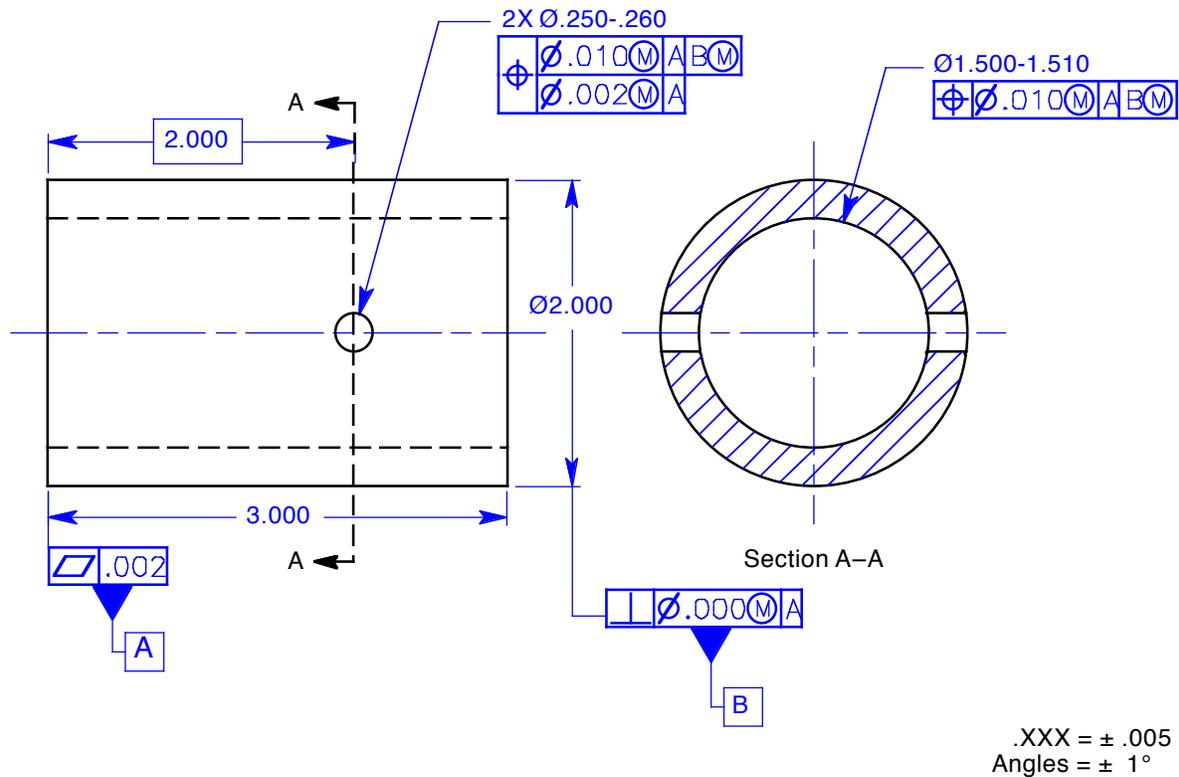
**Figure 9-13 A second method of tolerancing the part in figure 9-11**
