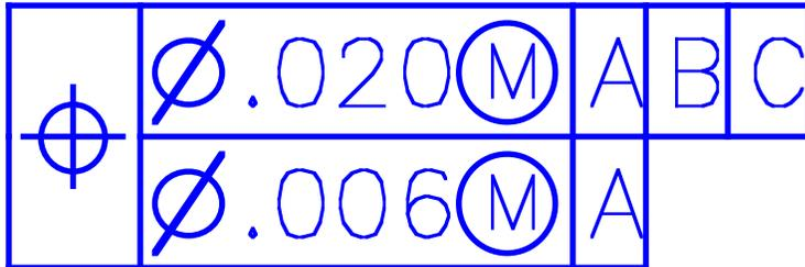
**Figure 8-14** The composite feature control frame.
