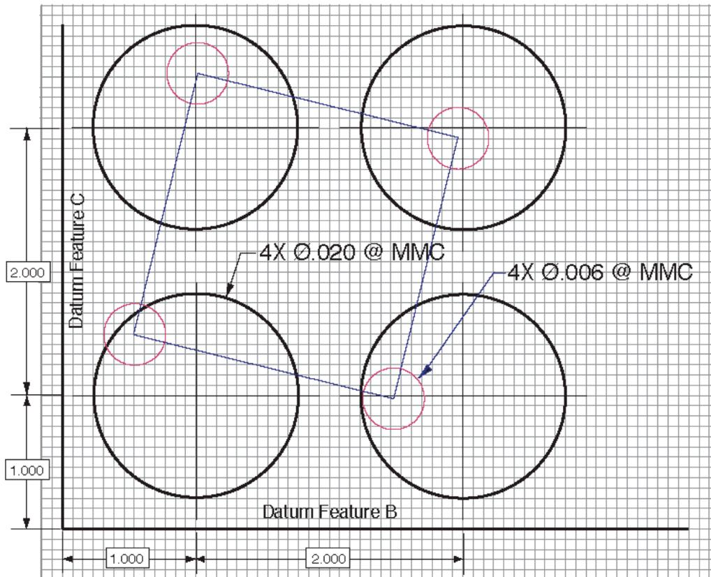
**Figure 8-15** The datum-to-pattern and feature-to-feature tolerance zone relationship for Fig. 8-13.
