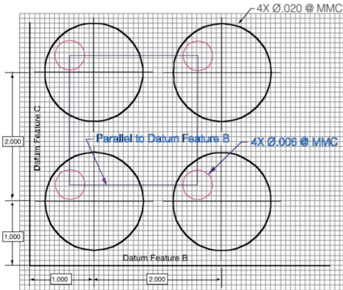
**Figure 8-17** The datum to pattern and feature-to-feature tolerance zone relationships for the drawing in Fig. 8-16.
