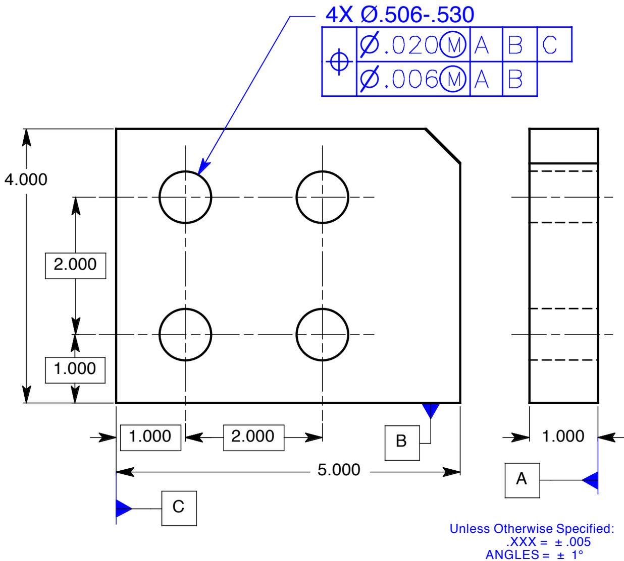
**Figure 8-16** A composite positional tolerance with datum features A and B repeated in the lower segment of the feature control frame.
