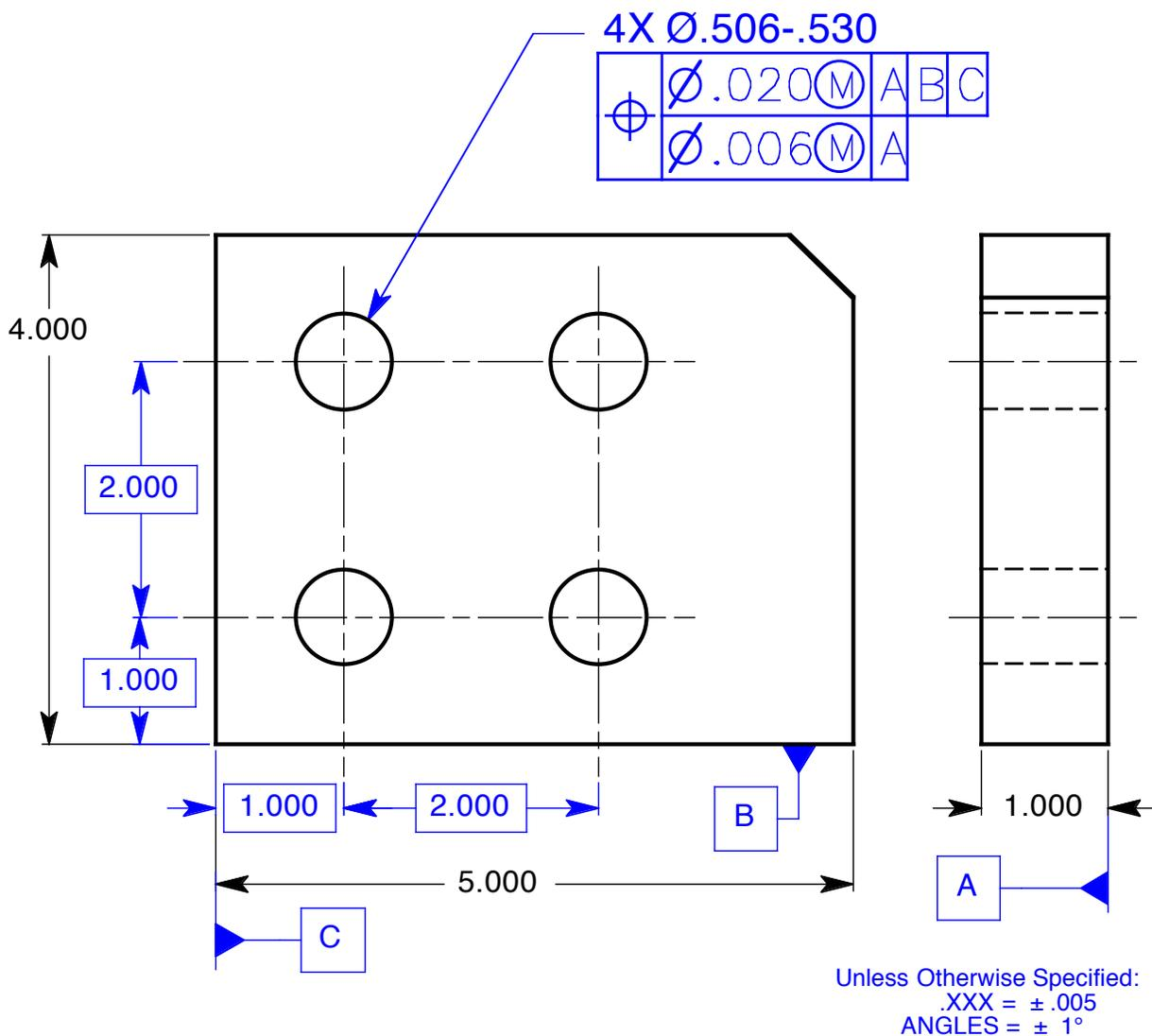
**Figure 8-13** A composite positional tolerance controlling a four-hole pattern to its datum features with one tolerance and a feature-to-feature relationship with a smaller tolerance.
