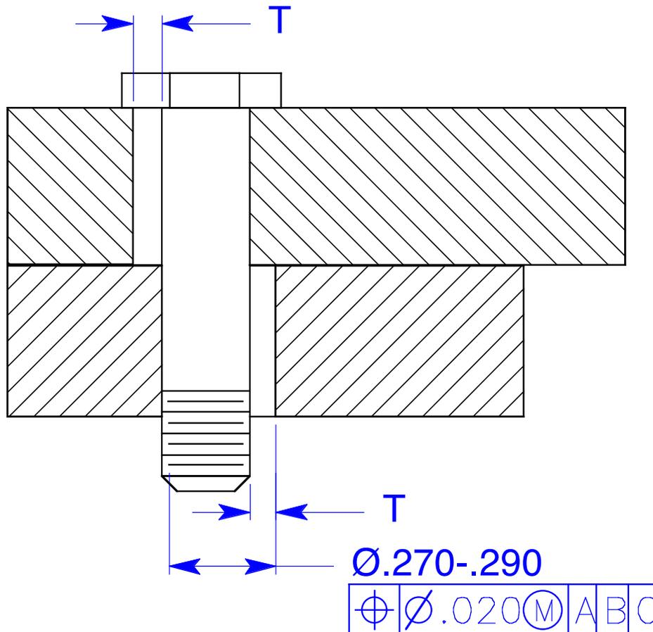
**Figure 8-1** Floating fastener
