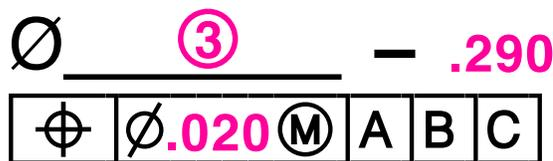
**Figure 8-2B** Dimension and tolerances for the floating fastener in Figure 8-1, the LMC hole size and the hole location tolerance are assigned
