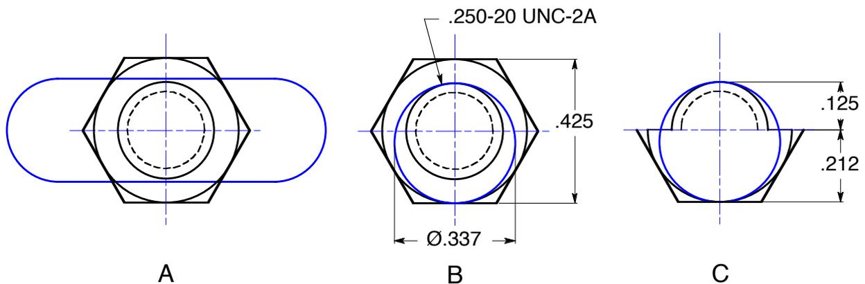
**Figure 8-3** Clearance hole least material condition diameter
