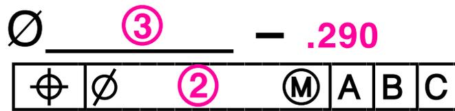
**Figure 8-2A** Dimension and tolerances for the floating fastener in Figure 8-1, the LMC hole size is assigned
