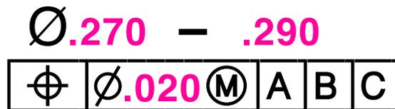
**Figure 8-2C** Dimension and tolerances for the floating fastener in Figure 8-1, the LMC hole size, the hole location tolerance, and the MMC hole size are assigned
