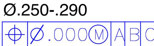
**Figure 8-4** A clearance hole with a zero positional tolerance at MMC.
