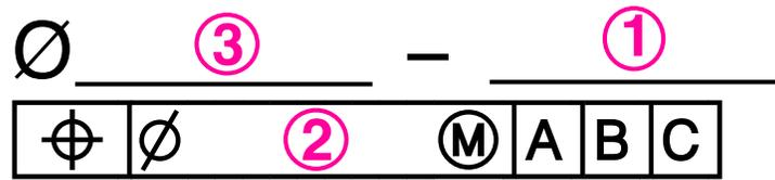
**Figure 8-2** Floating fastener dimension and tolerances
