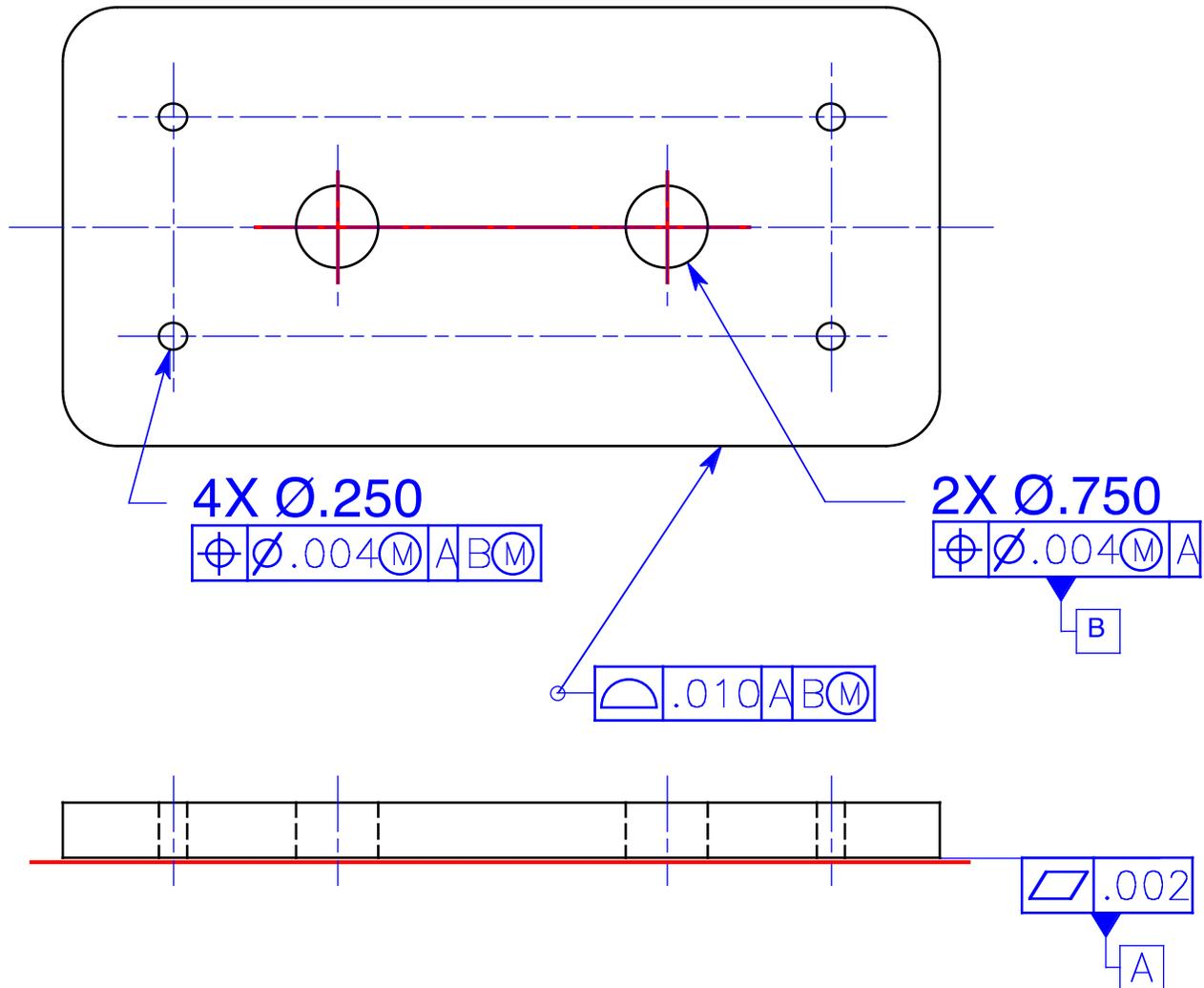
**Figure 14-14B A properly toleranced part shown in Fig. 14-14A**
