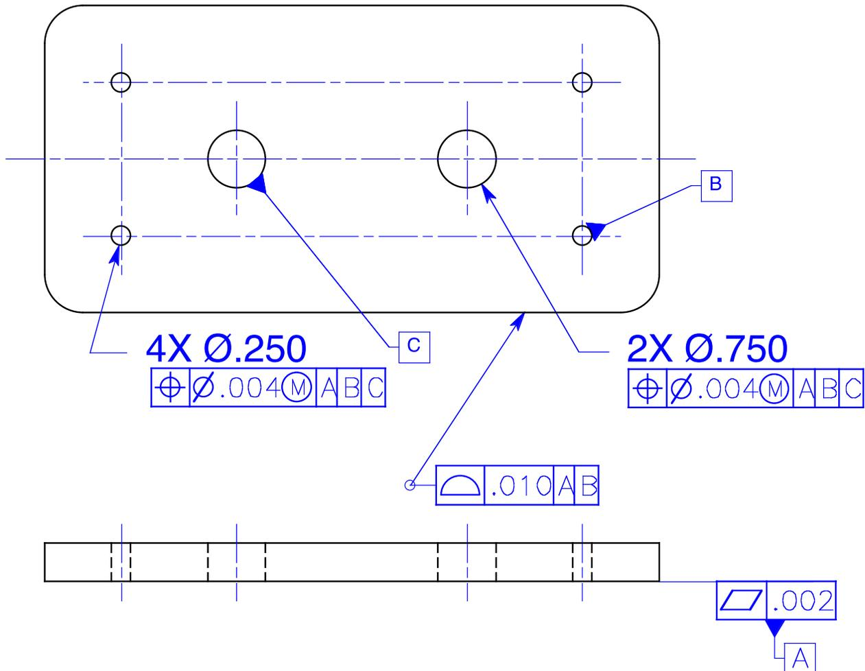
**Figure 14-14A The inappropriate use of datum features to control a pattern of features to another pattern of features**
