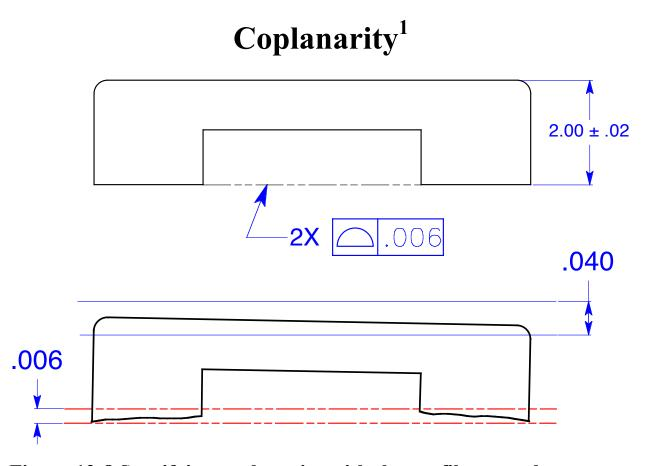
Figure 12-8 Specifying coplanarity with the profile control
