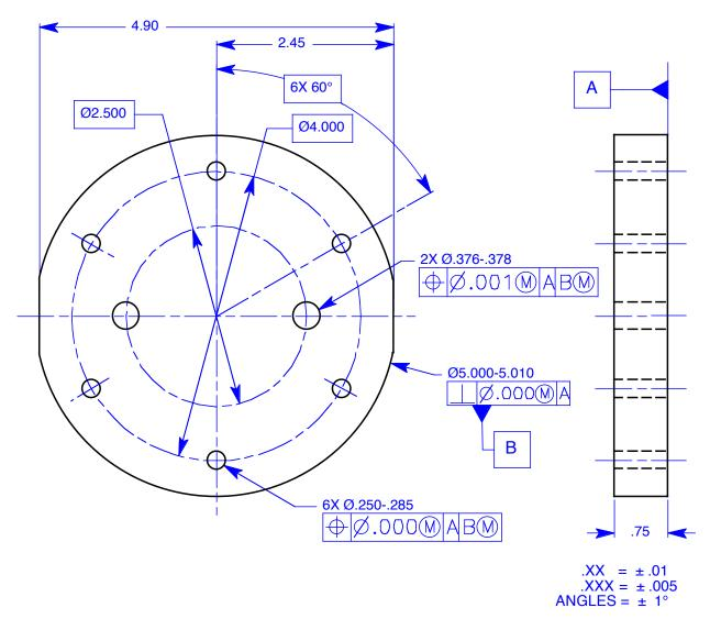
**Figure 2** A correct example of patterns clocked only to each other but free to rotate around the axis of datum feature B.
