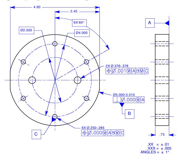
Figure 1 An example of patterns of features incorrectly clocked to a datum feature.
