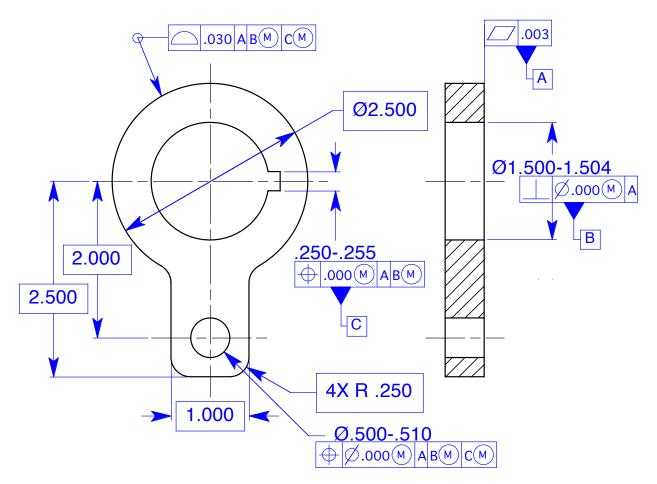
Figure 4 A good example of features clocked to a datum feature.
