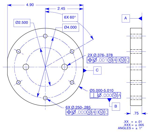
**Figure 3** A correct example of patterns of features clocked to each other and to datum feature C.
