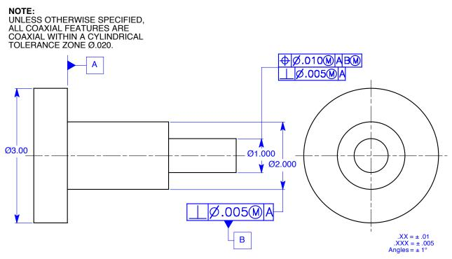
Figure 6-4B The properly toleranced part shown in Fig. 6-4A
